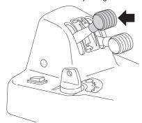
9 Set the required engine speed with the throttle control.
